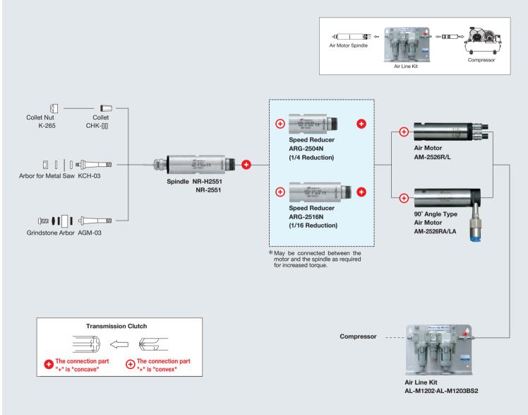
\*Do not exceed the maximum motor speed recommendation for the spindles. Excess speed will dramatically reduce bearing life.
